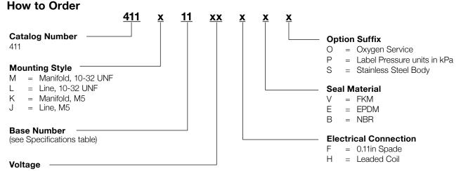
12 = 12 VDC 24 = 24 VDC 05 = 5 VDC 06 = 6 VDC
