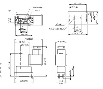
① 4 mounting holes, max. depth 7mm (0.276in), for self-tapping screw (type EJOT PT, K30)
