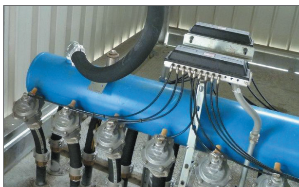
A two-stage pulse diaphragm valve. Threaded 2" connection with external control via pilot valve box.
