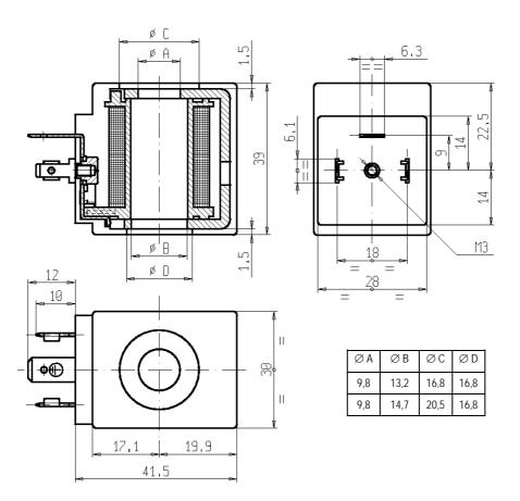
FEATURES - Windings made by class H (180°C) wires, vacuum impregnated by polyester resin then encapsulated in thermoplastic materials suitable for the insulation class of the product (see table below). Coil complying with VDE 0580 directive and 100% inspected.
