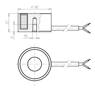
FEATURES - Series of solenoids with zinc plated steel body. Class F insulation (155°C) with class H wire (180°C). Solenoid complying with VDE 0580 directive and 100% inspected.
