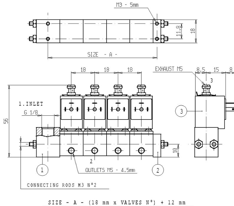
**FEATURES** - System designed to assemble banks of micro-solenoid valves with common inlet and single independent outlets. The feature consists of a through hole machined into the valve body that connects the common inlet of the plate group with the different components. The seal between the different micro-solenoid valves is guaranteed by a gasket supplied with the valve.
